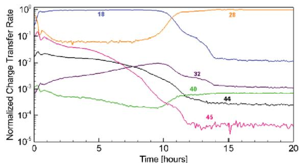
Figure 3: Residual gas analysis data for D-Mannitol in 2-Butanol and water<sup>2</sup>.
