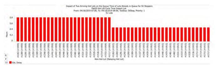
The above chart from FabTime's software shows another example. In this case, two hot lots arrive at the 5x Stepper tool group during the one-hour time period of the chart. Each of these lots jumps the queue and delays the roughly 25 lots already in queue by the hot lot process time ( $\sim 0.8$  hours for the first lot and  $\sim 0.5$  hours for the second lot).
