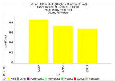
because it requires a particular tool, and that tool is down for parts. Putting the lot on hold makes it clear to the operator that nothing can be done with the lot at present, and the operator moves on to something else.
