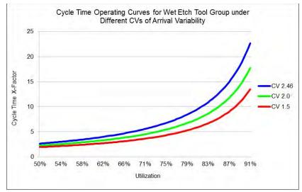
The other target that we had for building operating curves of real tool groups was to identify places where the cycle time in the fab is significantly higher than that predicted by the model. Where you see that happening, it's worth digging into the fab data to see what you might be missing:
