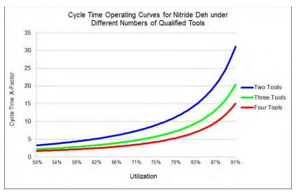
cycle time is still lower with the additional qualified tool. The resulting curves for two, three, and four qualified tools are shown to the right.
