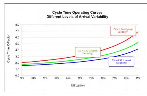
The difference in the curves would be the same if. instead of varying arrival variability, we varied process time variability, as those two are weighted equally in the formula. In either case, we can see that the impact of variability on cycle time through this one-of-a-kind tool is significant. The good news is that anything that we can do to reduce variability will tend to improve cycle times. Some concrete variability reduction suggestions (which have
