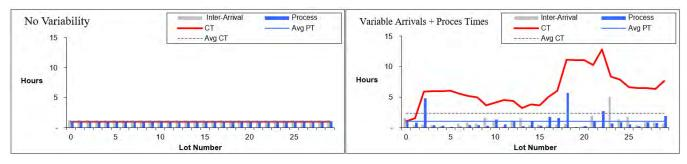
Running this simulation exercise at varying tool utilizations allows us to build an operating curve (a graph of cycle time x-factor vs. utilization) for this system. But there's an easier way to build the same operating curve using a simple queueing model. For a one-of-a-kind tool with no downtime under medium variability and independent arrival and process times (e.g., the tool does not get faster just because it is busier), the queueing formula is:
