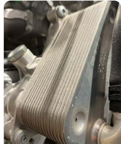
A plate heat exchanger in automotive application
