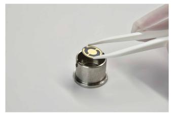
6 Replace the ceramic retainer by inserting it into the crystal holder at a slight angle and pressing down gently. Avoid using excessive force when handling the ceramic retainer to prevent breakage. Avoid rotating the ceramic retainer after installation to prevent scratching the crystal electrode.
