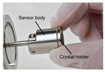
3 Insert the tapered end of a crystal snatcher (PN 008-007) into the ceramic retainer as shown below and apply a small amount of pressure. This locks the ceramic retainer to the snatcher and allows the ceramic retainer to be pulled straight out.
