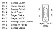
**Note** - If you are replacing the analog output version of the Granville-Phillips<sup>®</sup> 354 Micro-Ion<sup>®</sup> module, simply plug your existing cable into the BAG302 module 9-pin D-sub connector marked "Analog". See the following page if you are using the RS485 (with setpoint Relay) version of the Granville-Phillips<sup>®</sup> 354 Micro-Ion<sup>®</sup> module.
