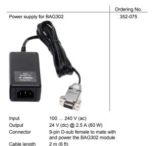
This variation of the power supply may be used when an AC plug that is not listed above is required. The conventional IEC60320 AC power entry receptacle allows use with any user supplied AC mains power cord set available worldwide.
