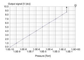
A) >10 V (dc). See the conditions listed above which will cause the output to switch to >10 V (dc). These conditions are above.
