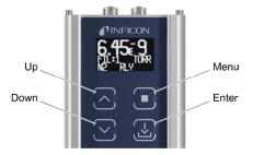
There are four soft-keys located on the front panel, below the display. These keys are used to select and program the various functions available. During programming of the BAG302, the display will identify what each function key represents.
