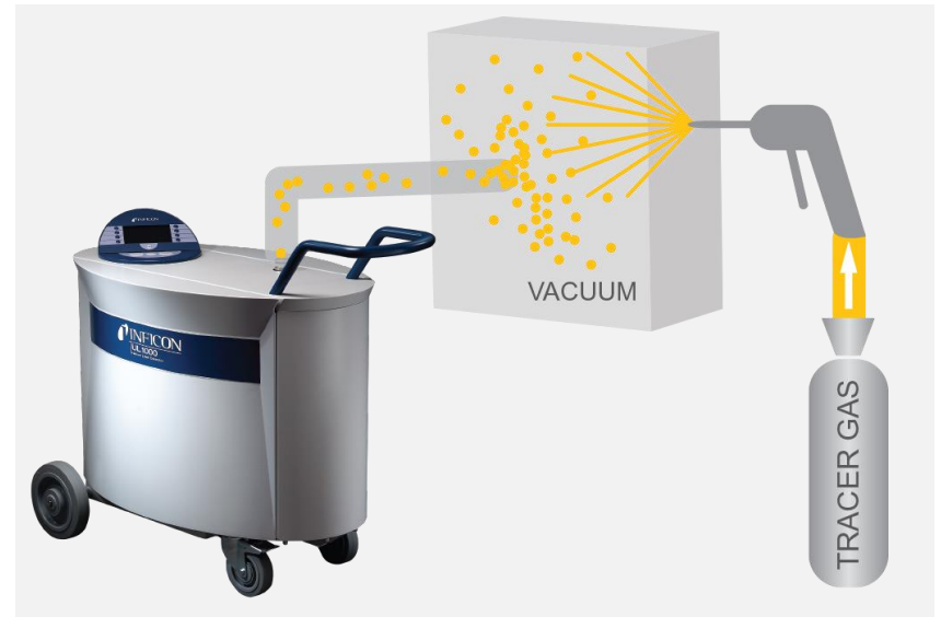
Spraying leak testing
