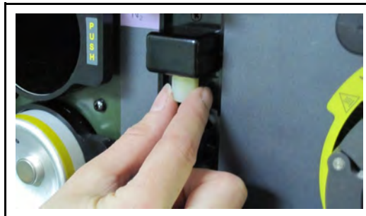
Figure 3-41 Loosening the Concentrator Nuts
