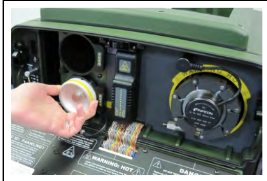
Figure 3-11 Internal Standard Installation Verification
