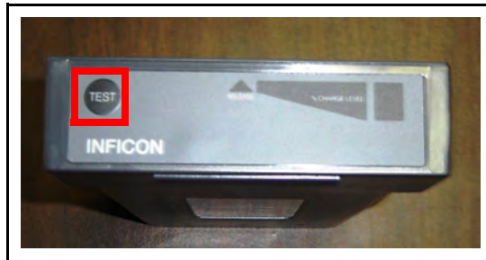
Figure 3-33 Battery TEST Button
