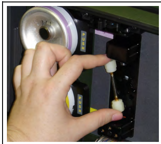
Figure 3-46 Placing Concentrator in the Bottom Elbow
