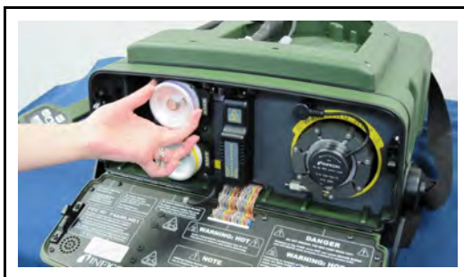
Figure 3-15 Carrier Gas Installation Verification
