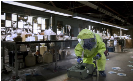
HAPSITE CDT portable chemical identification system identifies and quantifies narcotics, explosives and toxic industrial chemical threats
