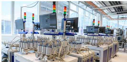
Long-term test system for vacuum gauges, Balzers (LI)
