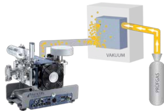
Diagram of the vacuum method – with a vacuum in the test chamber.
