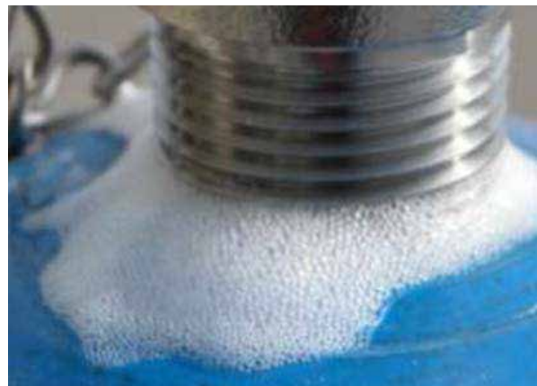
Foam test on a threaded connection.
