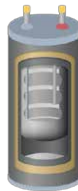
Picture of a storage-in-storage system.
