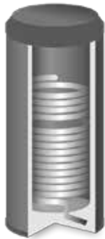
Picture of a storage heater.
