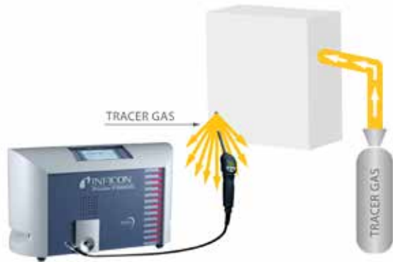
Diagram of the sniffer leak detection – with a manual sniffer tip.
