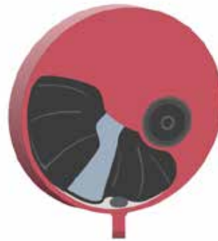
Schematic illustration of an expansion vessel.
