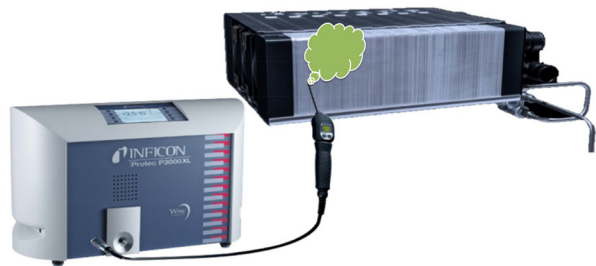
Sniffer test on a fuel cell stack.
