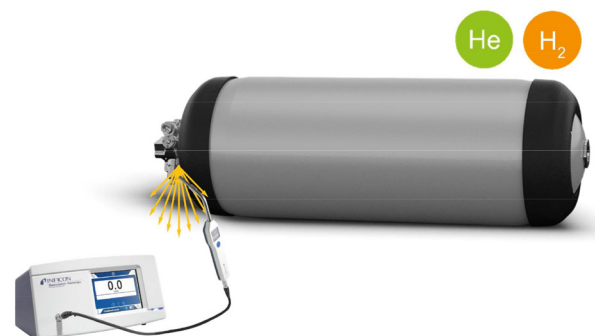
Sniffer leak detection on the fittings of a hydrogen tank.
