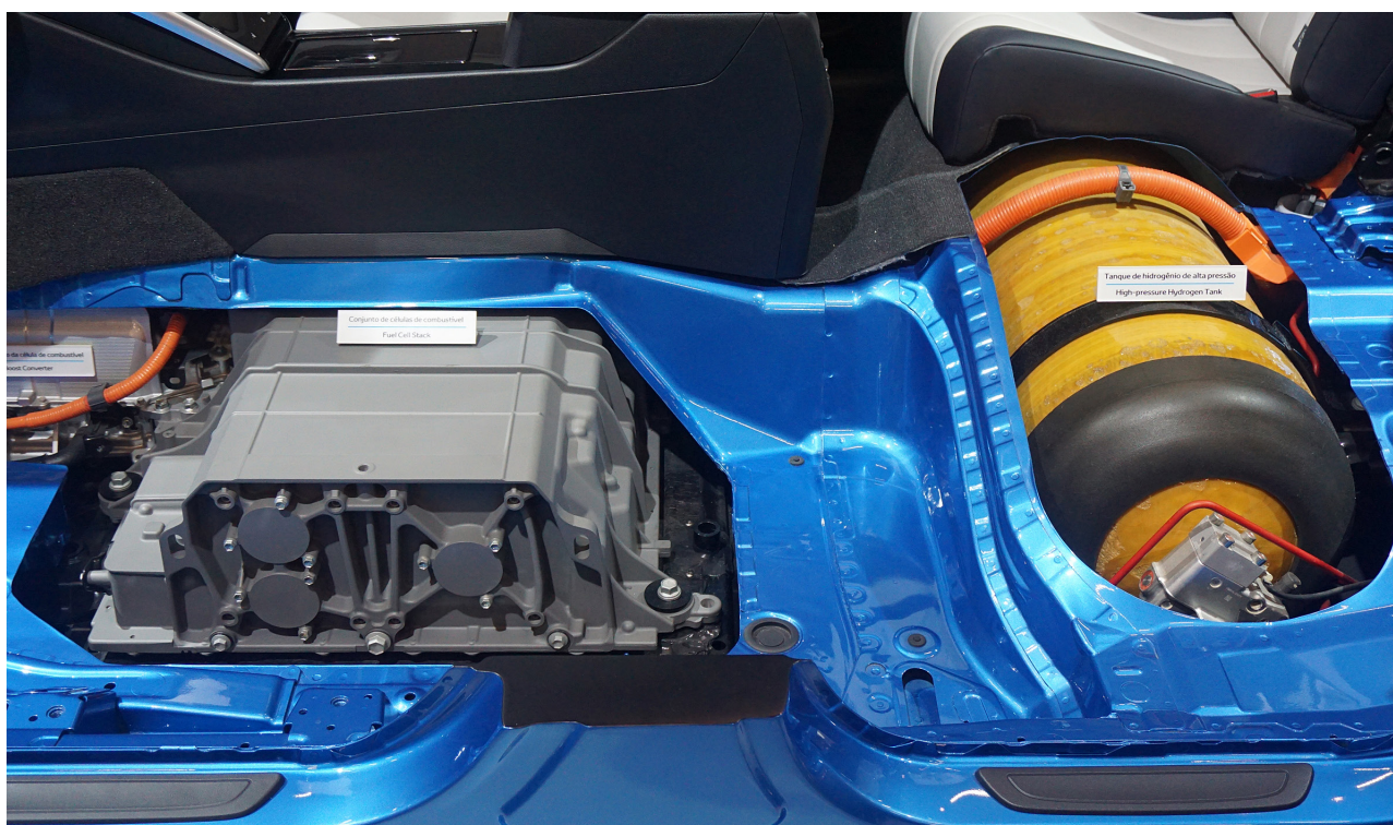
Hydrogen tank installed in a Toyota Mirai.
