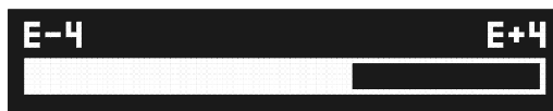
Bar graph. The symbol of the corresponding measuring channel flashes (e.g. A1).
