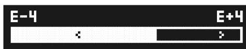
Bar graph with setpoint. The symbol of the corresponding measuring channel flashes (e.g. A1).
